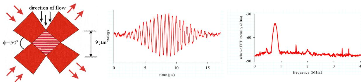
Figure 2. Laser Doppler Velocimetry. (left) crossed laser beams (centre) light scattered by probe particles (right) Fourier transform yields local velocity in probe volume.
