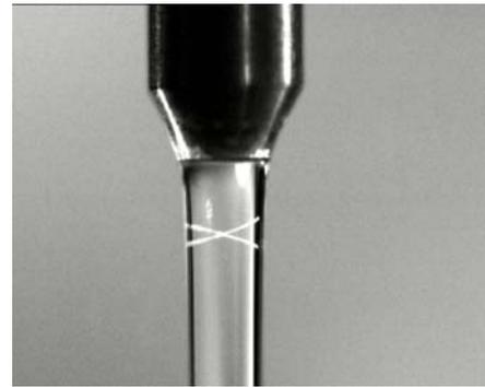
Figure 1: Aqueous jet emerging from 0.8-mm radius SS nozzle. The crossed laser beams are for laser Doppler velocimetry.
